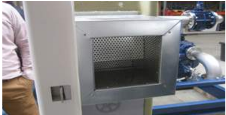
Air vents are also acoustically treated
