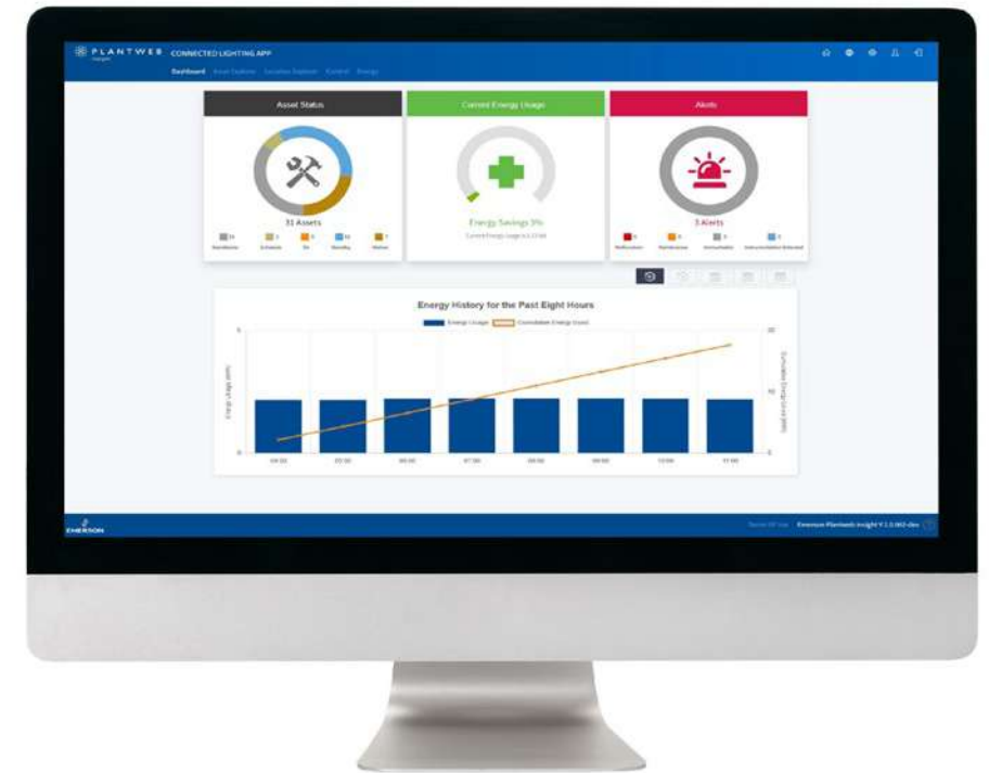
Figure 17: The Plantweb Insight Connected Lighting application monitors individual fixtures, and it aggregates system performance to capture overall energy use.
